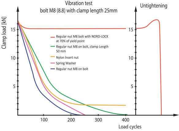
The test diagram shows the bolt tension during vibration testing of some common fasteners. Most commonly used locking devices show limited performance when exposed to vibration.
